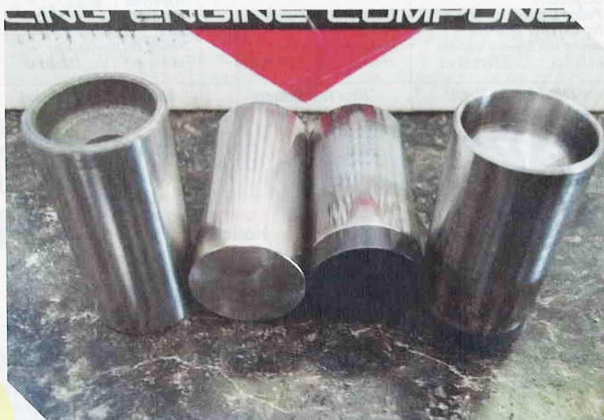
We ran all of our cams with Schubeck composite-faced lifters and set the valve spring load to meet their requirements. By using "ceramic" lifters, this meant that we eliminated the need to break in several different camshaft and lifter combinations, and to keep installing and removing the inner valve springs for proper break in. Unfortunately, Schubeck Lifters are no longer in business.
